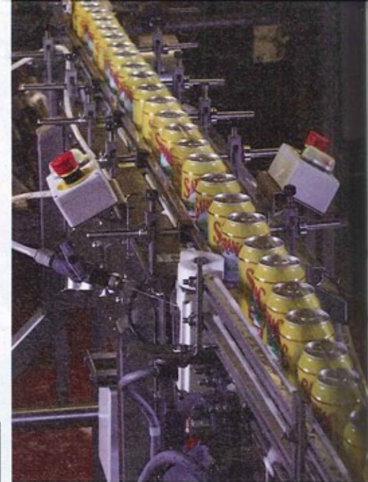
Cans of Saranac beer line up on the conveyor before entering the checkweigher to ensure fill accuracy.
