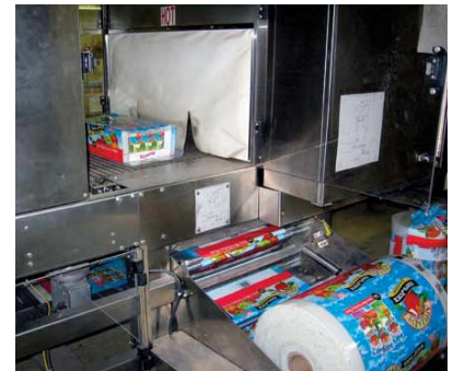
TRAYPACK DISCHARGE. The brightly decorated film, a 2-mil high-density polyethylene, is printed flexo in seven colors.
