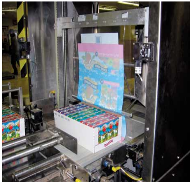
SHRINK WRAPPING. Film is applied in register by this single-curtain shrink wrapper/tunnel combination system, whose small footprint was among the features so attractive to CEA.
