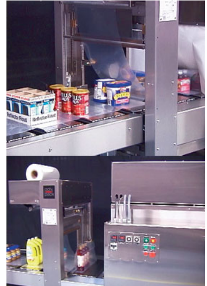
The conveyor carries the packages through a curtain of film, which is pulled across the tops and bottoms of the packages as they travel through the film.
