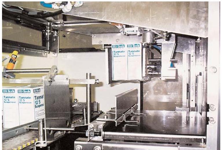
Quick-change Pick & Place grippers can stack & rotate collated products.
