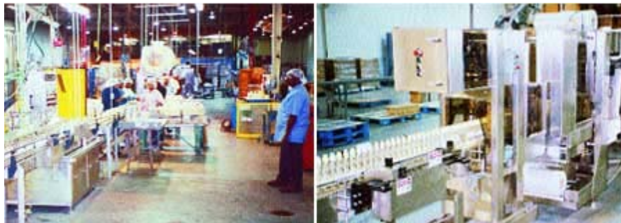
Hair and body wash bottles, left, single file from a rotary filler and capping/pump placing station to the bundling machine infeed, right. They're grouped into two lanes, oriented into two six-packs and wrapped.
