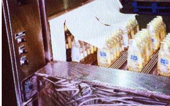
Multipacks of bottles emerge from the bundling machine's shrink tunnel, in two sets of six, before they exit the machine. The six-pack bundles are then loaded by operators into shipping cases erected on a new case former also recently installed on the line. The line outputs approximately 26 bundles, or 160 bottles per minute.
